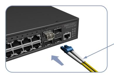
Connect 62.5/125 or 50/125 multimode or 9/125 single-mode fiber with LC connectors.
